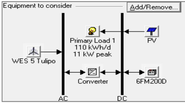
Figure 10. Designed system in HOMER
