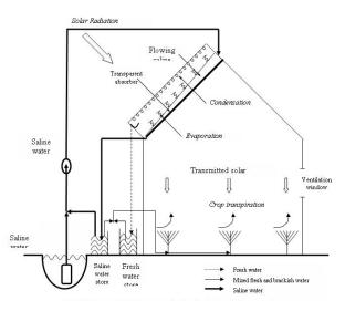
Figure 3. System principle for water desalination integrated in greenhouse roof
