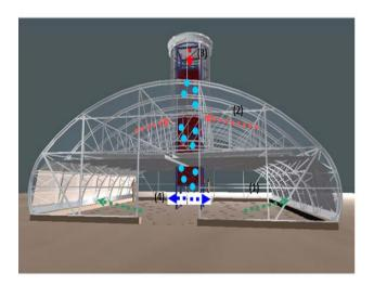
(1)Humid air from greenhouse through evapo-transpiration process); (2) Ascension of heated air to the tower –trough secondary collector; (3) Cooled air to fall back to the greenhouse through condensation on heat exchanger; (4) Irrigation to plants
