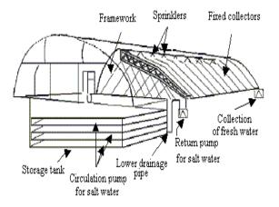
Figure 2. Greenhouse with solar desalination (M.Dument and M. de Cachard, 1978, Grenoble, France
