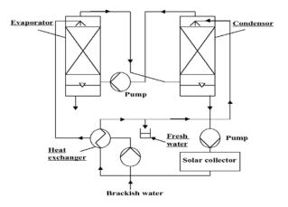
Figure 6. System principle for solar desalination plant using heat pipes collectors
