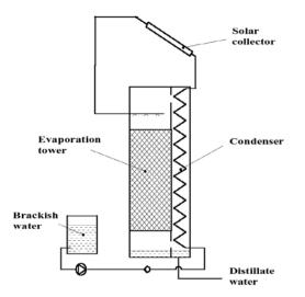
Figure 7. Solar multiple condensation evaporation cycle process with flat plate solar collectors
