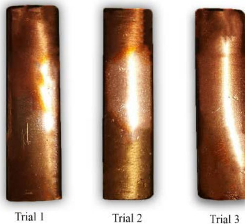
Figure 2. Post copper corrosion test images of copper strips (Heated from Mixed Biodiesel at 120°C for 3 hours ± 5 minutes)
