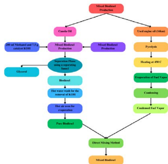
Figure 1. Schematic Diagram of Mixed Biodiesel Production
