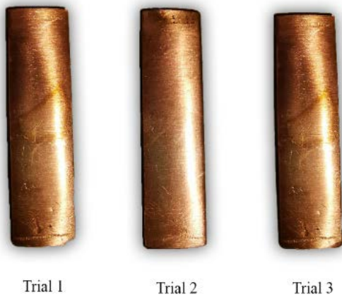
Figure 3. Post copper corrosion test images of copper strips (Heated from Commercial Diesel at 120°C for 3 hours ± 5 minutes)
