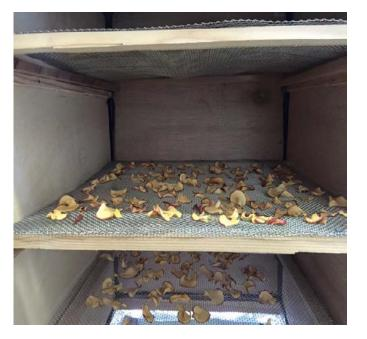
Dried apples in the drying chamber (before dryer modification)
