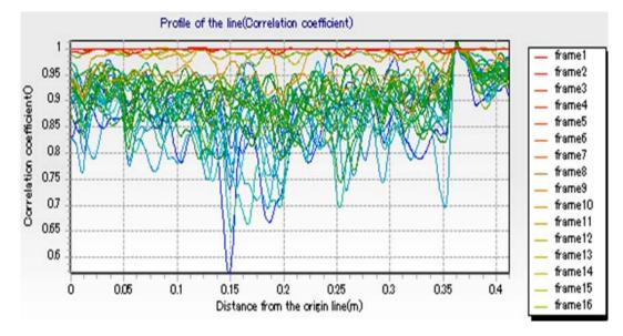
Figure 8. Graph of Correlation Coefficient across the drying chamber
