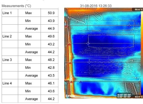
Figure 11. Thermal image showing temperature variations across 4 different sections
