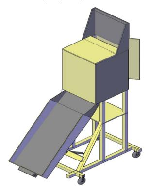
Figure 1. Existing solar dryer design
