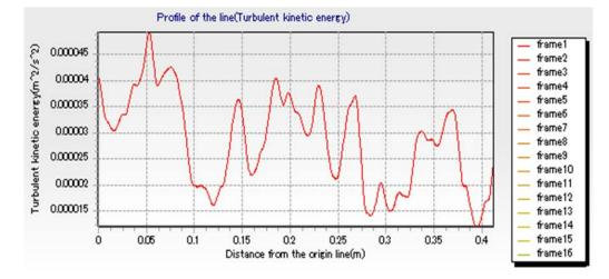
Figure 9. Graph of Turbulent Kinetic Energy across the section (between tray 2 and 3)
