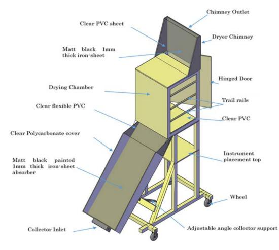
Figure 2. Modified Design solar dryer for PIV study
