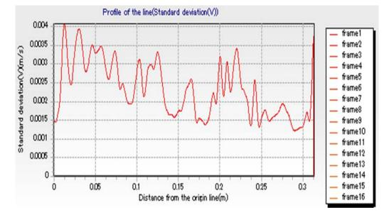
Figure 10. Graph of standard deviation of velocity within frames across the section
