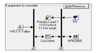
Figure 10. Designed system in HOMER
