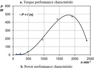
Figure 13. H-Darrieus wind turbine performance characteristics
