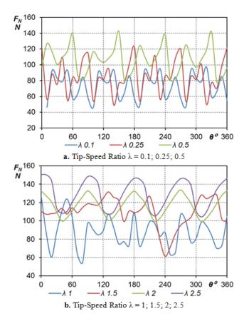
Figure 17. Normal force distribution for a full turbine revolution
