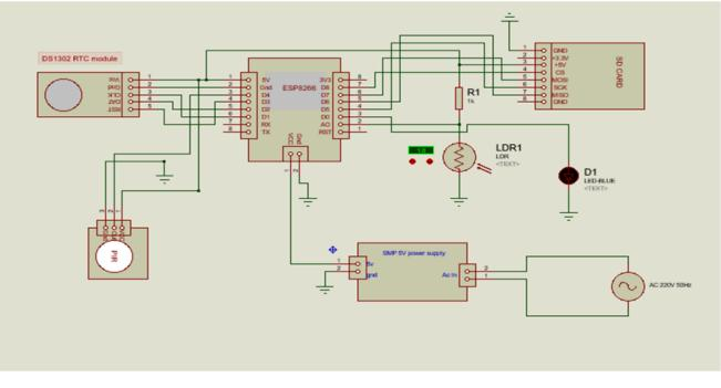
Figure 3. Circuit Diagram for Sensor Node 2
