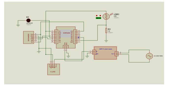
Figure 2. Circuit Diagram for Sensor Node 1
