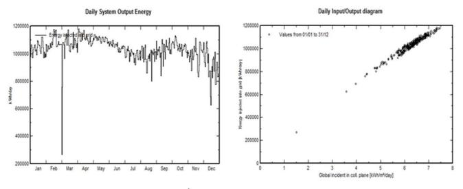
Figure 6. Daily input/output diagram (kwh/m²/day) & Daily system output Energy (kwh/day) of Al-Shuaiba PV project
