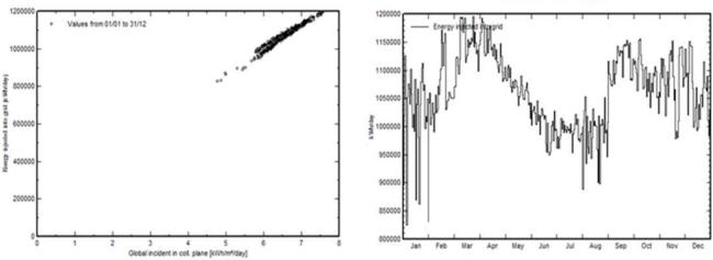
Figure 10. Daily input/output diagram & Daily system output Energy of Al-Shuqiq PV project
